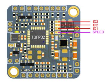
Jumper ID3 is responsible for entering compatibility mode. If it is open, the CAN Switch Board can be configurable using Light Client software (speed, base ID, rotary switch configuration), and the device transmits data using the new V3 data format. The default speed is 500 kbps, and the base ID is 0x640.
