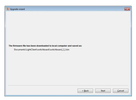
Next, press the *Start* button to upgrade the firmware. During the upgrade process, do not turn off your PC or interrupt power to the device!
