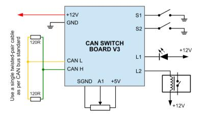
The CAN (Control Area Network) bus was developed for communication in automotive applications. Its construction is very simple (only two wires) and its immunity to interference is very high. In modern vehicles, dozens of different electronic modules may communicate via the CAN bus.
