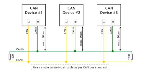
In automotive applications, typical data rates on a CAN bus are 1 Mbps, 500 kbps and 250 kbps. The following conditions must be met for each speed:
