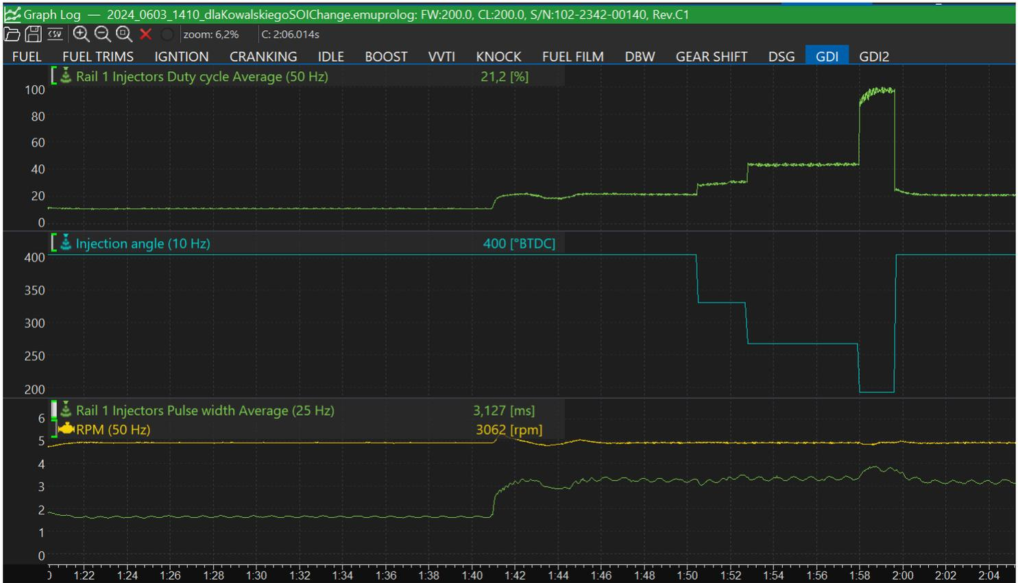
**Pressure target - Effect on injector duty cycle**
