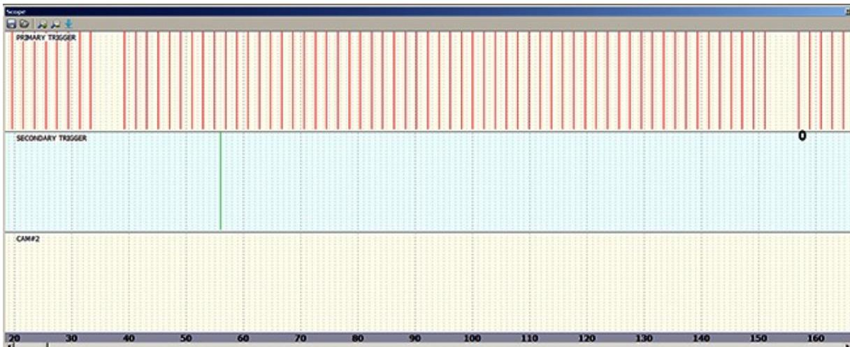
Toothed wheel 60-2 located on crankshaft, 1 tooth cam sync
