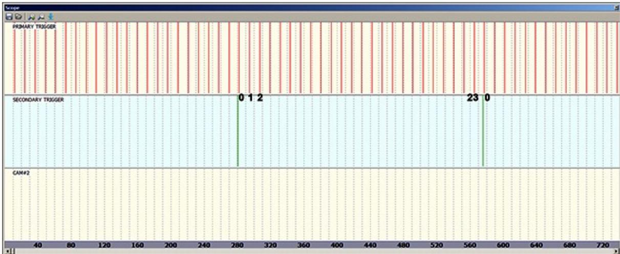
Toothed wheel with 12 evenly spaced teeth located on crankshaft, 1 tooth cam sync
