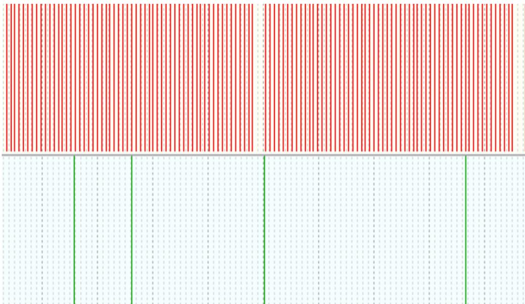
Correct scope for camshaft trigger wheel signal
