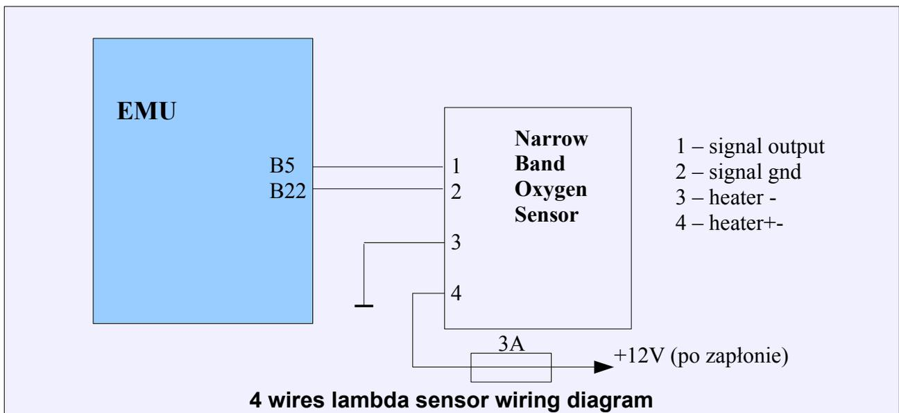
In the case of using 1 wire oxygen sensor the voltage read by EMU for stoichiometric mixture is 2.95V, for the 4 wire sensor it is 0.45V.
