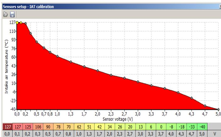
Using the wizard we can use the predefined sensor, or create its characteristic, providing the sensor resistance for 3 known temperatures. The highest difference of temperatures is recommended in the wizard (these data can be found in the car's service book or can be collected with ohmmeter in 3 different temperatures)
