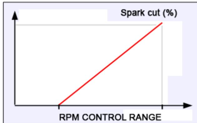
Interpolation of spark cut value in the control range region
