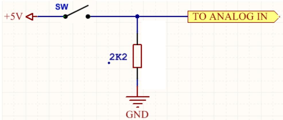
In the case of Analog input #x option, the activation is performed if the voltage on analog input is greater than 4V
