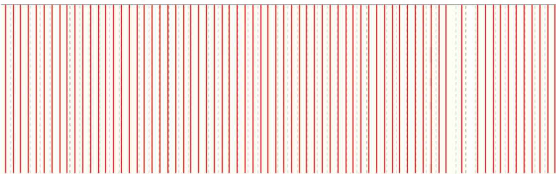
Incorrect scope for 60-2 trigger wheel
