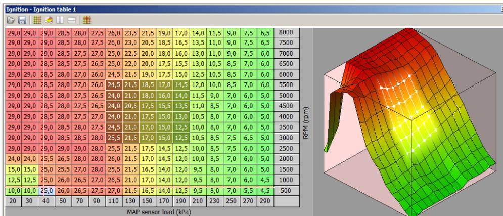
*Ignition angle table* is the main table used for ignition angle advance. The resolution of this table is 0.5 degrees. Positive values indicate a spark angle before TDC, negative values mean the spark angle after TDC.
