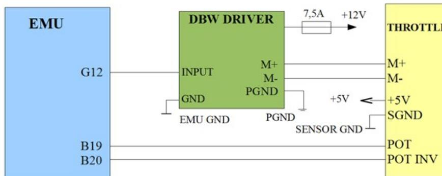
The diagram shows how to connect the module DBW, EMU and the electronic throttle
