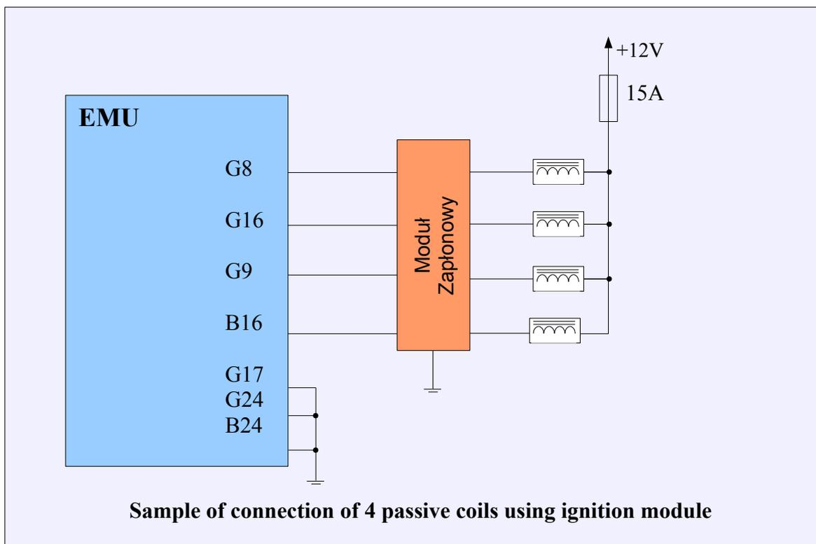
In case of active coils or using ignition modules, there is a chance to connect two coils or module inputs to one ignition output in order to do wasted spark ignition.
