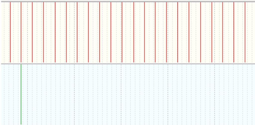
Incorrect trigger edge setup for multitooth
