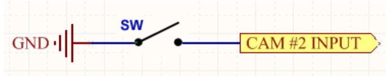
There is an option to connect switch to *CAM#2 input*. To use this option internal pullup of CAM#2 input must be activated in *Ignition / CAM #2 options*
