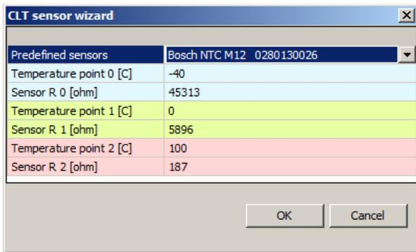
**Predefined sensors** – names of predefined sensors. In case of choosing the „User defined” sensor it is possible to add temperature values and resistance of own sensor.
