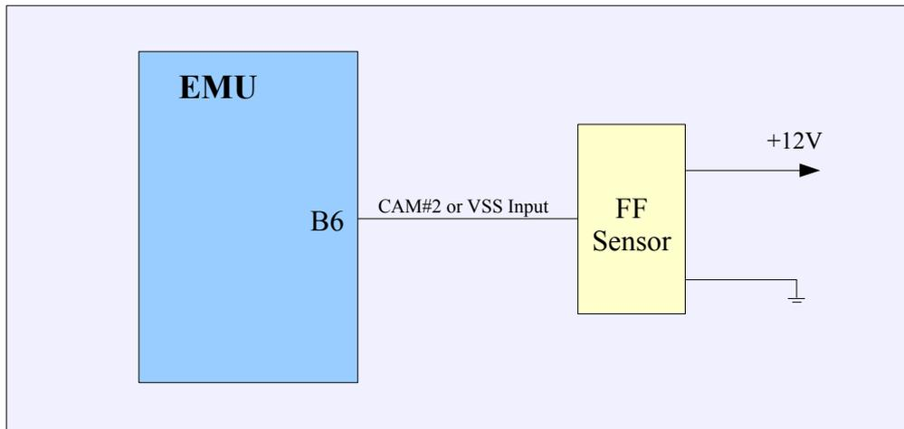
The *FlexFuel* sensor should be connected to the CAM#2 input or to VSS input if the CAM#2 input is used for a camshaft position sensor. To activate the *FlexFuel* sensor, the *Enable FlexFuel* parameter should be checked and *Table switch mode* should be set to *FlexFuel* blend in options menu *Other/Tables switch*.
