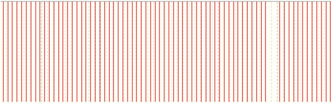
Correct scope for 60-2 trigger wheel
