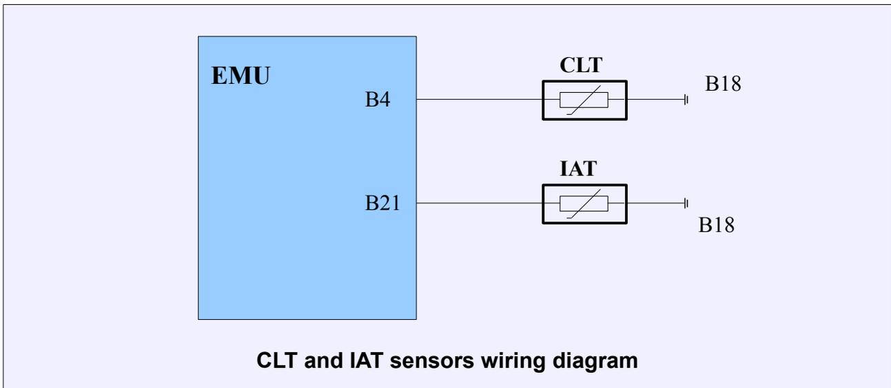
IAT and CLT sensor calibration takes place by using 2D tables, respectively, *IAT Calibration* and *CLT Calibration*. This table defines the divider's voltage created by the sensor and built in the EMU pull-up resistor corresponding to the given temperature. In order to facilitate the sensor calibration, you should use the wizard.
