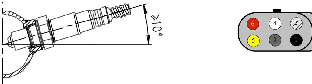
**Installation of the lambda probe in the exhaust system. Pionout of the LSU 4.2 connector**
