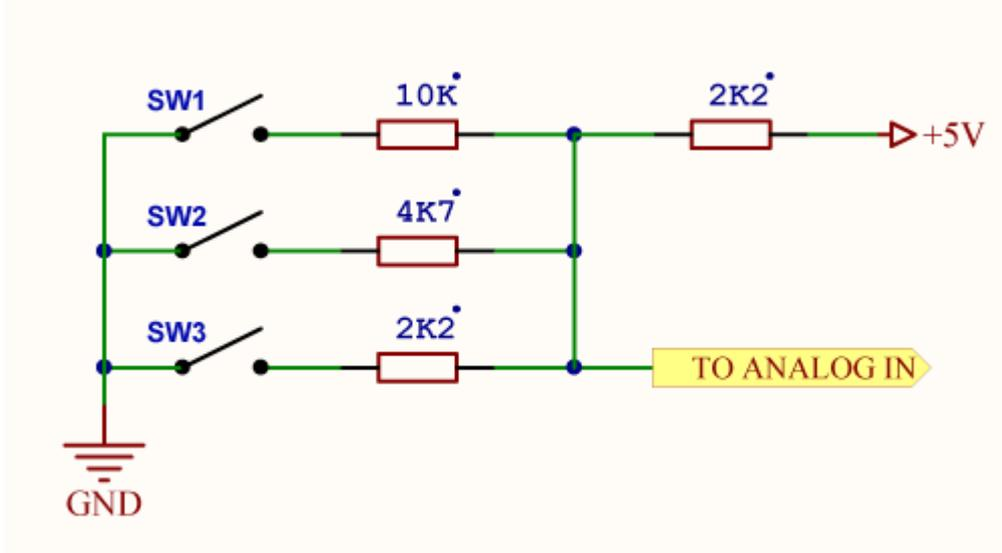
The MUX Switch function allows to connect up to 3 switches to one analog input. More information can be found in *Sensors setup / MUX Switch* section
