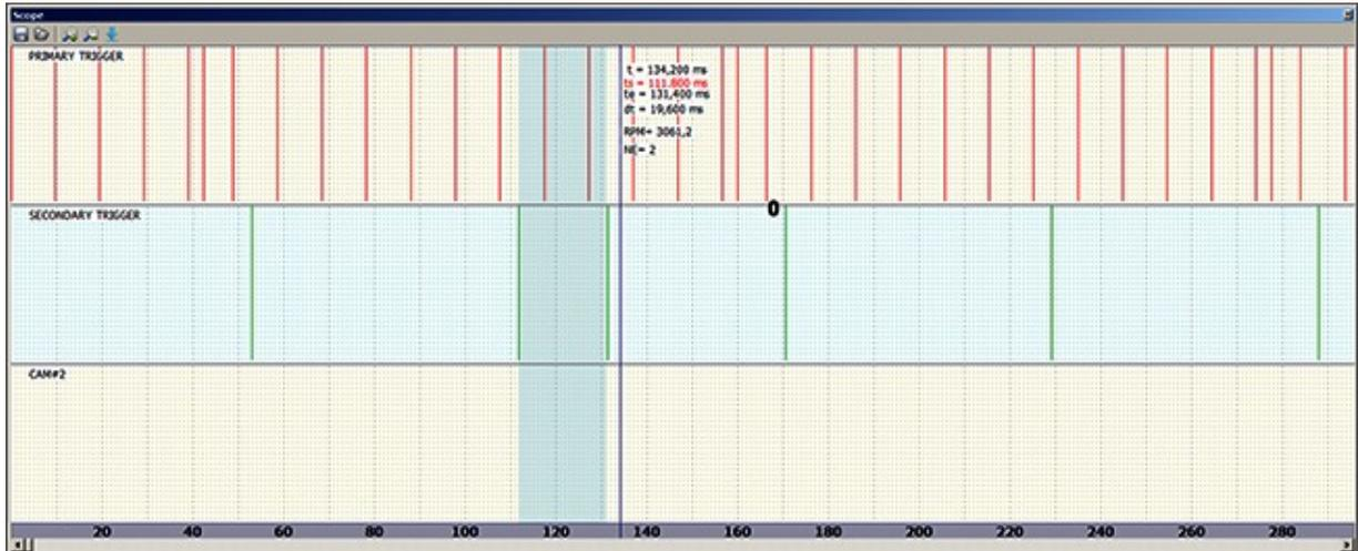
Toothed wheel 12+1 located on crankshaft, camsync N+1. N+1 cam decoder.
