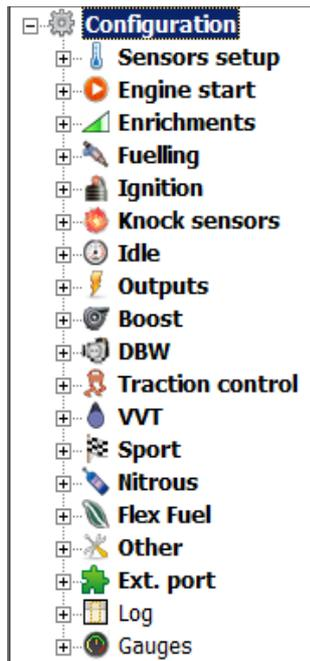
On the left there is a list of all available EMU functions grouped in functional blocks. Depending on firmware version there could be different set of functions. By expanding functional group user can access parameters and tables.
