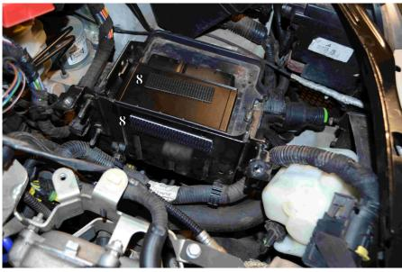
Repeat operation with adapter. Apply 3M dual lock tape on stock ECU mounting, and adapter itself. Check proper side of the adapter (8).
