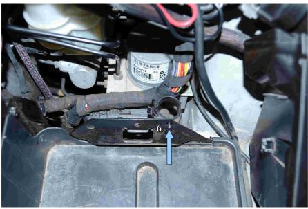
Remove plastic mount holding stock wiring harness by pressing out bolt (6).
