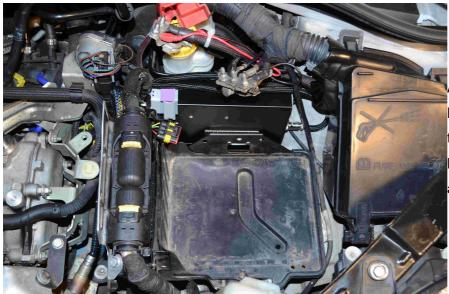
Attach EMU behind battery holder. arrange harnesses no to tight. Connect OEM harness ECU plugs to adapter.
