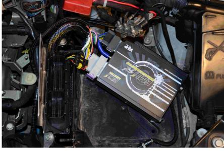
Connect EMU to wiring harness. Connect CAN BUS communication to extension port. Connect supplied vacuum hose from intake manifold to EMU ECU (cut vacuum hose to fuel pressure regulator and connect with Tjoint).
