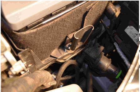
Remove windshield washer fluid reservoir and unscrew M8 nut holding fluid reservoir mount (4).
