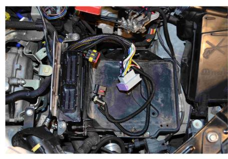
Connect supplied wiring harness to adapter, and mount adapter in stock ECU place. Mount heat shield and tighten M6 bolts (3) 12Nm.
