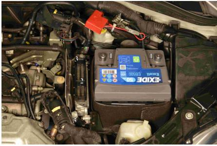
Remove positive and negative terminal of the battery (1).
