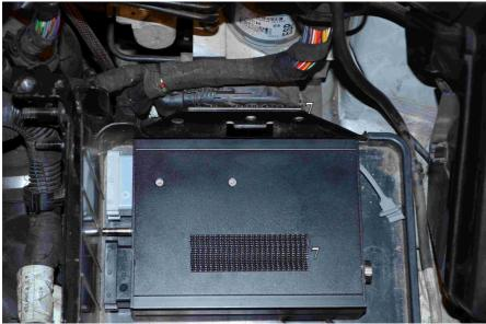
Apply 3M dual lock tape on EMU ECU and metal mounting element (7).
